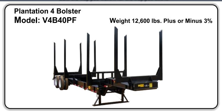
The New Viking Plantation 4- Bolster combines every manufacturing quality that makes up the viking name. Designed to haul a variety of harvested timber. Capacity: 80,000 lb. GVWR.
