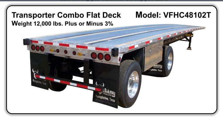
The "Transporter Combo Flat" from Viking Specialized Trailers combines the quality and durability that goes into every Viking trailer. Aluminum crossmembers, outriggers, side rail, bulkheads and flooring come together to make our lightest Flat Bed trailer produced. This trailer was designed to last and allow you to haul the most. The Viking Specialized "Transporter Combo Flat" new ideas and innovation at work for you. Capacity: 80,000 lb. GVWR.
