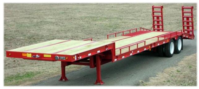
The Equipment Transport trailer was designed to deliver two 4-wheel machines on site. It also has the ability to haul fuel and other items needed in the field on the upper deck. The two lift transport is a must have when getting equipment delivered on site. Three wheel machines can also be hauled with the addition of a third ramp. Capacity: 80,000 lb. GVWR.
